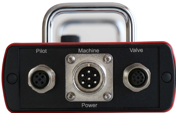
Figure 8: Connector view of the test device ValveExpert Checker 2.3. See Tables 3 and 4 for Pin assignment.
